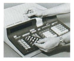
With a choice of modules. One, three different, or ... you can use any combination of three modules at the same time. Each gives you special functions, plus more memory. Each block contains its own read-only-memory (ROM). Here are the blocks currently available.
