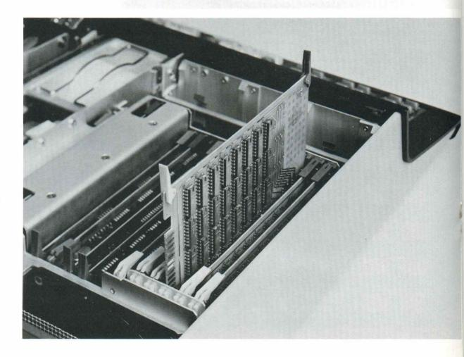
An expandable internal memory for speed. Using advanced MOS/LSI technology, the 9820 has a fast read/write memory for you to use. Basic capacity is 173 registers, but you can expand to 429 or a maximum of 1,447. These numbers translate into the capability to solve 71 simultaneous equations.
