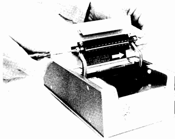
Figure II-9. Removing the Old Lamp.
