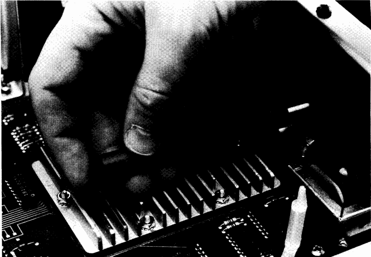
Figure 3-2 Adjusting the +12 Volt Supply
