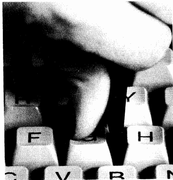
Figure 2-12 Removing a Key Cap
