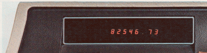
The optional light-emitting-diode (LED) display allows continuing verification and aids in editing during long problems. It may be used with the printout or without it (saving paper).
