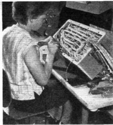
Left to right: the Honeywell Golden Gnat miniature rate gyro and its rotor; wiring up the BG-158 computer in its "jeep can"; and testing the autopilot
