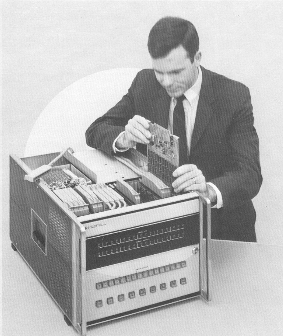
Interface cards are installed or moved by top access. Device cable attaches directly to the interface card.
