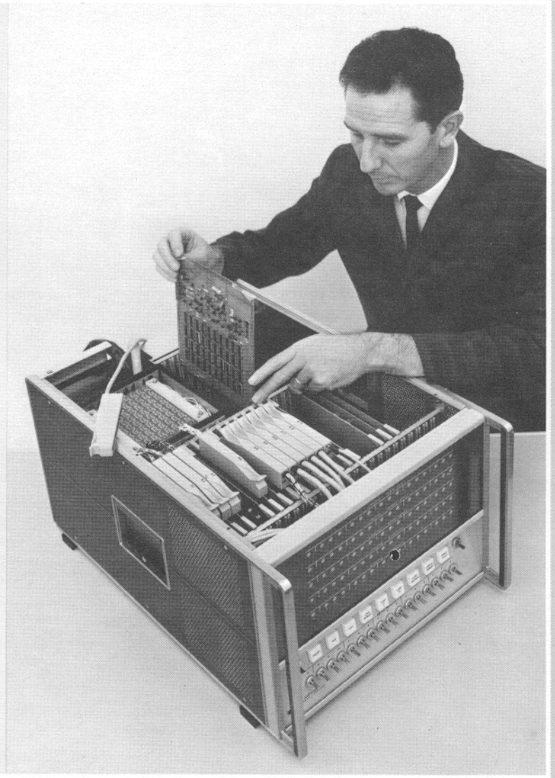
Interface cards are installed or moved by top access. Device cable attaches directly to the interface card.
